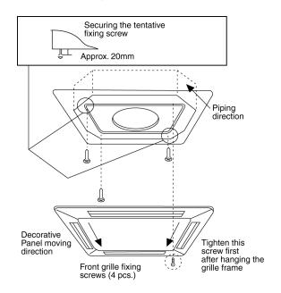
3 Fit the decorative panel and ceiling wall together and confirm no gap in between. Readjust indoor unit height, if there is a gap between ceiling wall and decorative panel.
