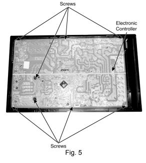
$\Delta$  Caution! When handling electronic controller, be careful of electrostatic discharge.
